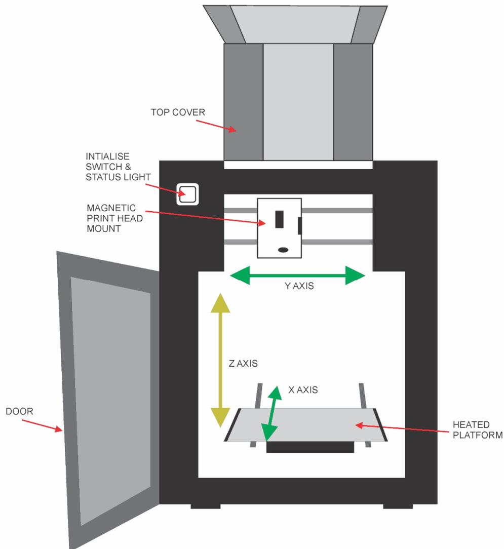
Figure 2. Back view of printer
